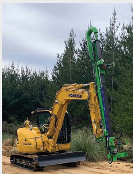
Pruning machine in development by Hudson Clearwood Ltd
