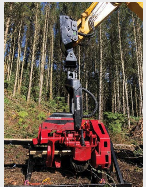
Steelwrist SQ80 quick coupler connected to a Waratah 624 processor (note processor cradle)
