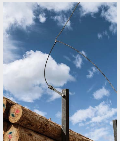
Prototype Trinder Engineering chain placer mounted on a log trailer
