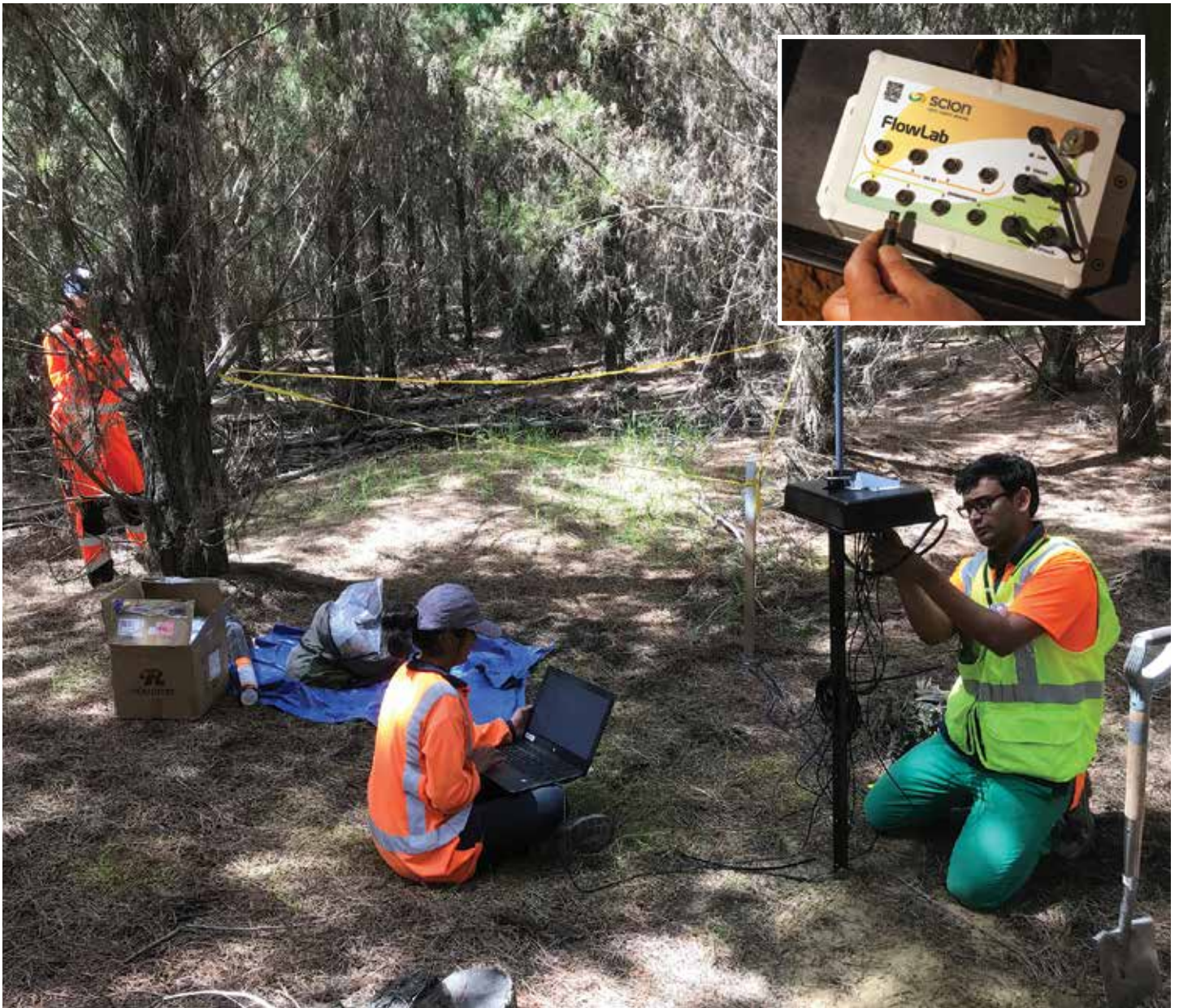
Members of the Scion Flowlab team installing a sensor at a Forest Flows monitoring site. Inset: The Flowlab wireless data logger
