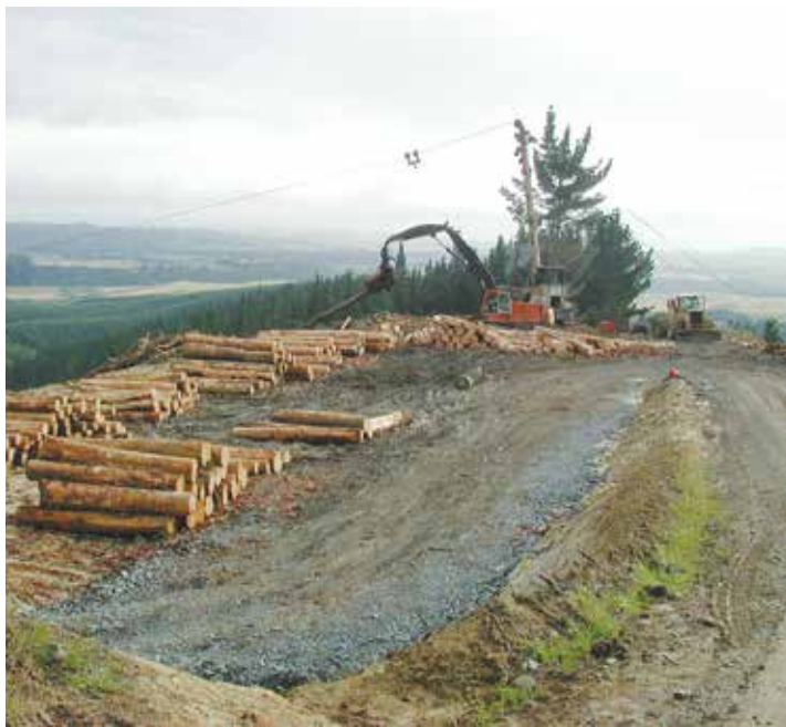
Spur road landing
