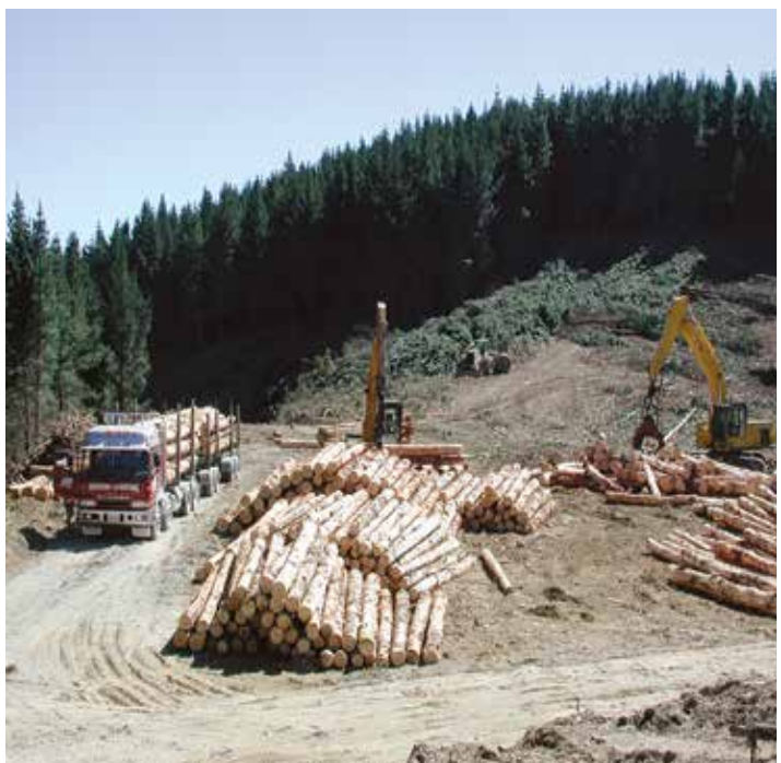
Roadside landings provide a clear separation between landing activities and the road, but can require more effort to reach logs stacks when loading out
