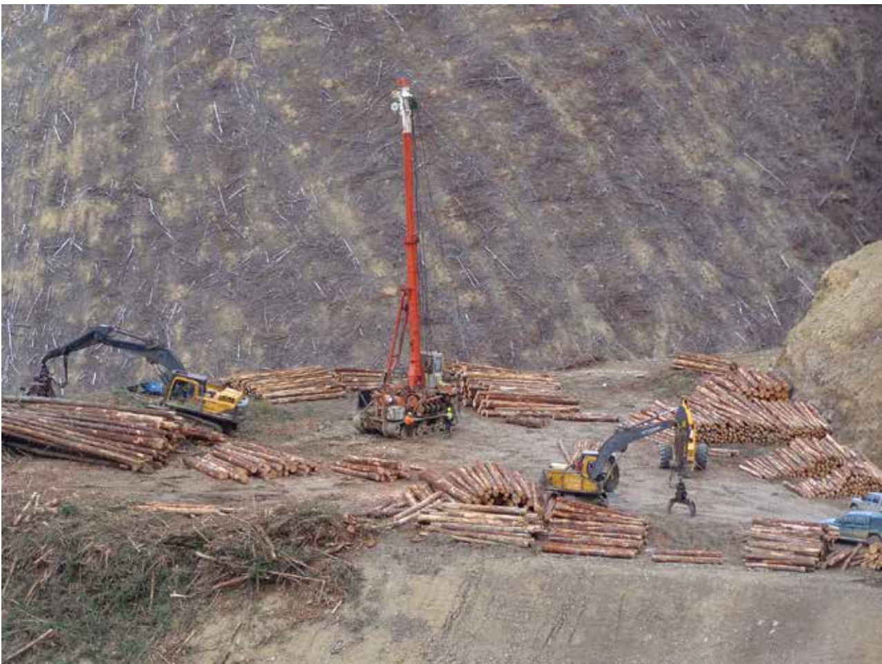
A cable yarding operation working on a landing
