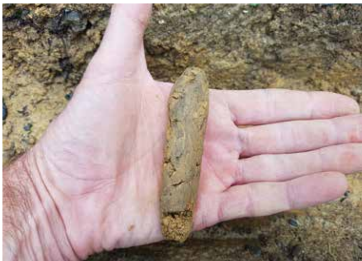
Left: The process of rolling a worm is a simple test for clay content. Right: The pat and tap test for silt
