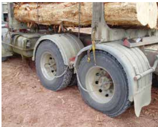
Central tyre inflation on the drive wheels
