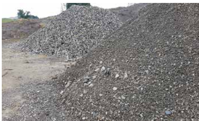
Crushed concrete may be a non-traditional alternative where there is a close source. Two screened grades can be seen
