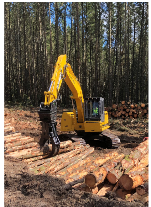
The Ensign 1770L fixed top continuous rotating grapple allows a skilled operator to carry out all log handling operations including sorting, stacking, loading, and shovel logging
