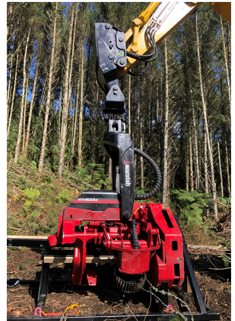
The Steelwrist SQ80 Quick Coupler attached to the Waratah 624C grapple processor
